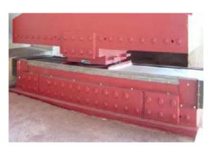
Fig.20 : Sliding isolator type SI
