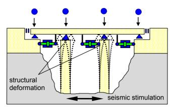
Fig. 6: Bridge with active MSTU's during seismic event
