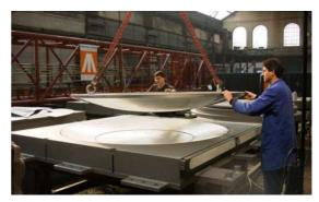
Fig.21 : SI - sliding isolator for 130,000 kN load (SLS)
