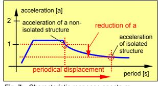
Fig. 7: Characteristic response spectrum of a bridge
