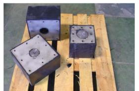
Fig.16: Rubber isolators with lead core (LRB)
